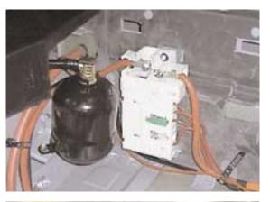
The main fuse box is located inside the glove box above a hinged panel. This places the power distribution close to the main electronics carrier behind the glove box.
